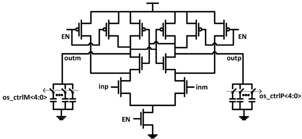
Fig. 7. Schematic of the SAR ADC comparator with offset calibration.
