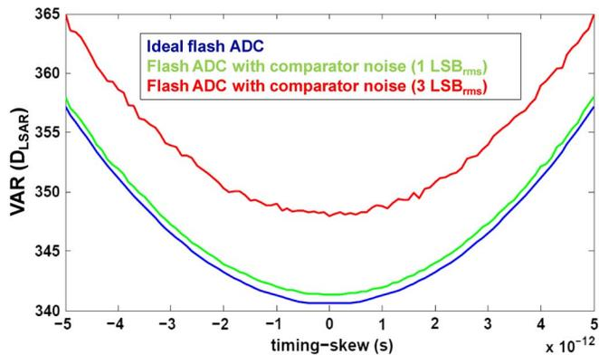
Fig. 12. Behavioral simulation result with comparator noise in the flash ADC.
