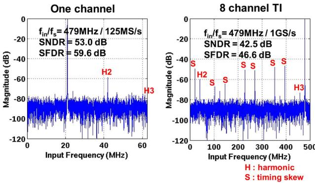
Fig. 16. Measured spectrum before calibration: single channel result (left) and time-interleaved result (right) with a Nyquist rate input signal at 479 MHz.
