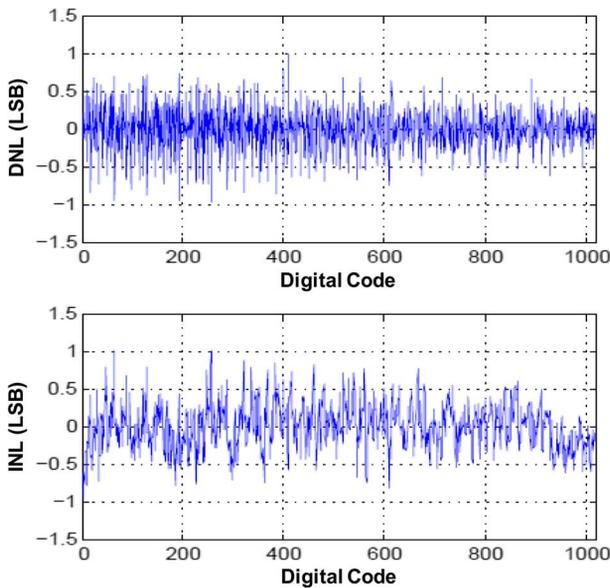
Fig. 19. Measured INL/DNL of the ADC.
