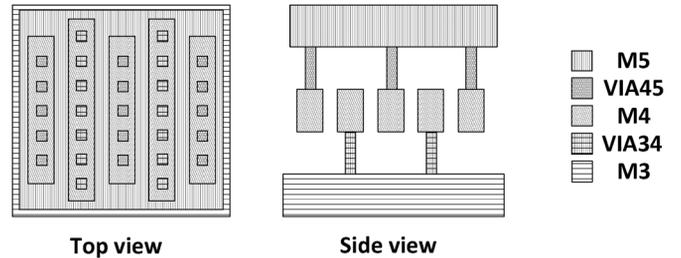
Fig. 6. Custom-designed unit capacitor.
