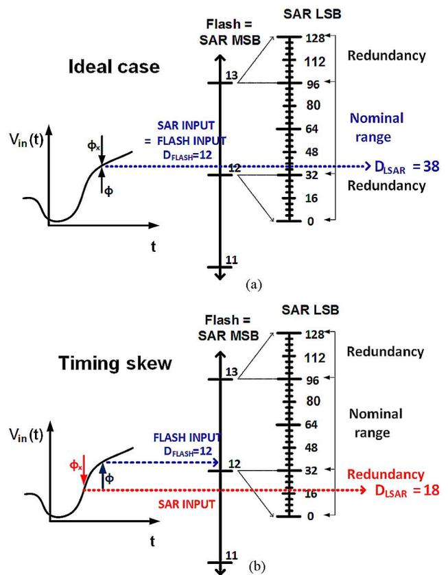
Fig. 8. Conceptual diagram of the ADC operation. Top: ideal case without timing skew. Bottom: realistic case with timing skew.
