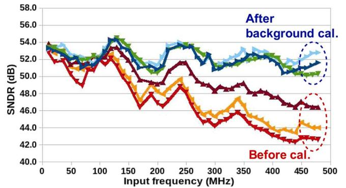
Fig. 22. Measured SNDR versus input frequency from three different chips.
