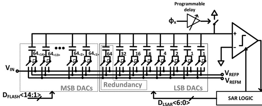
Fig. 5. Implementation of the 10 bit SAR ADC (a single-ended version is shown for simplicity).
