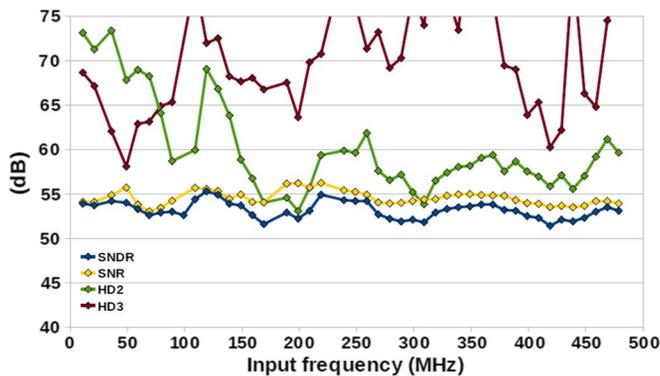
Fig. 21. Measured SNDR/SNR/HD2/HD3 versus input frequency of a single channel.
