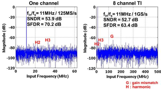
Fig. 15. Measured spectrum before calibration: single channel result (left) and time-interleaved result (right) with a low frequency input signal at 11 MHz.
