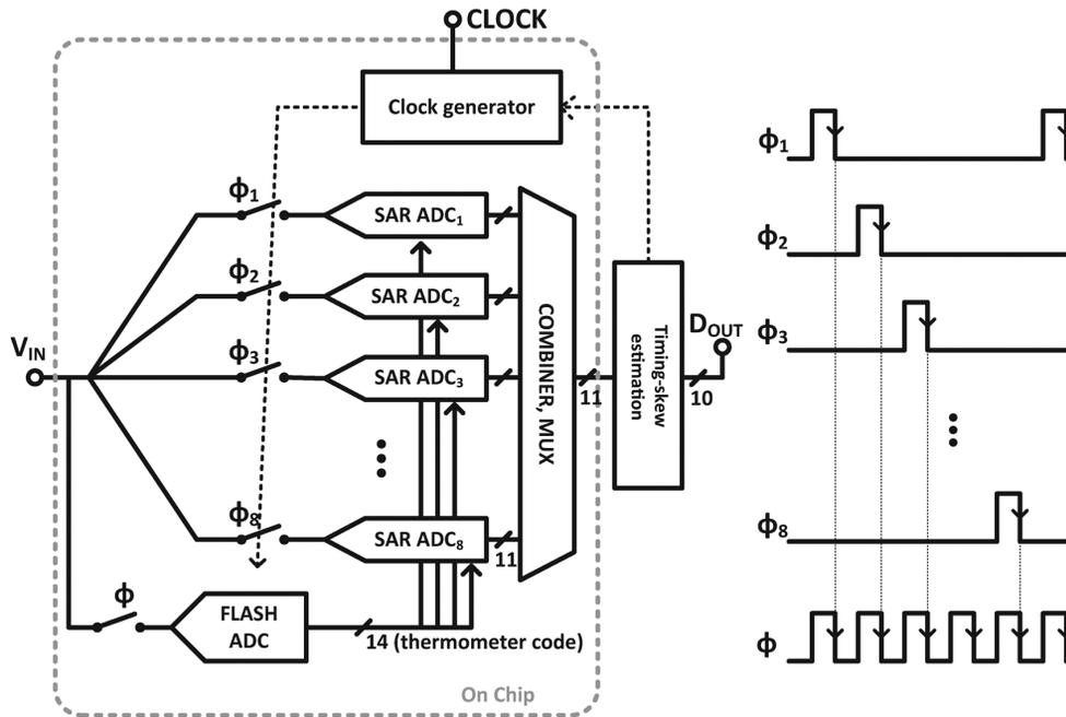
Fig. 1. Block diagram of the proposed TI SAR ADC.
