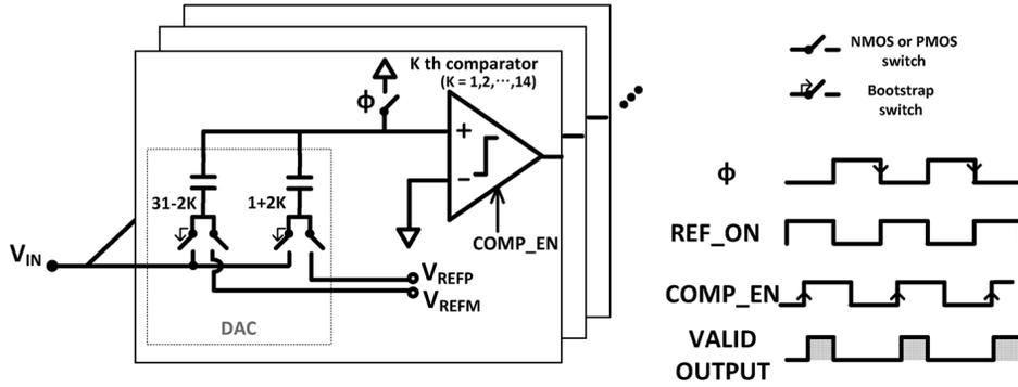
Fig. 4. Implementation of the 4 bit flash ADC (a single-ended version is shown for simplicity).
