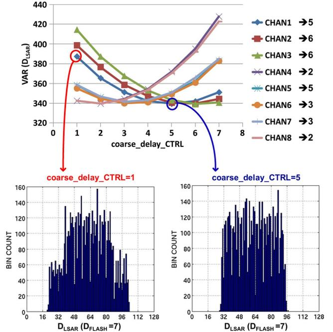
Fig. 17. Measured variance of  $D_{LSAR}$  against coarse delay control code of SAR ADC sampling clock (top) with the examples of the  $D_{LSAR}$  histogram for channel 1 (bottom).
