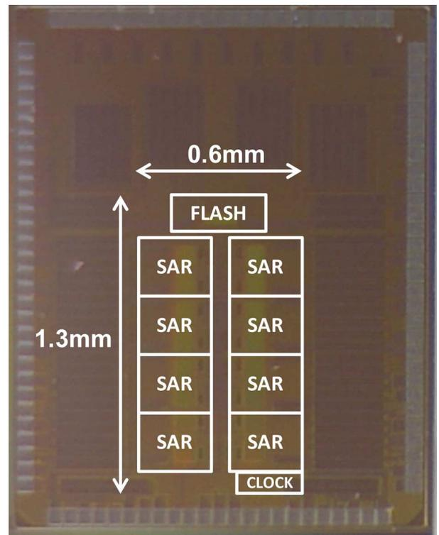
Fig. 23. Die photograph of the time-interleaved SAR ADC.
