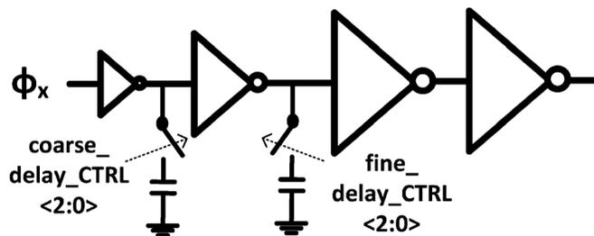
Fig. 3. Schematic of programmable delay block.
