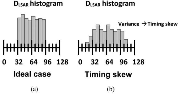
Fig. 9. Examples of the  $D_{LSAR}$  histogram (a) without timing skew and (b) with timing skew.
