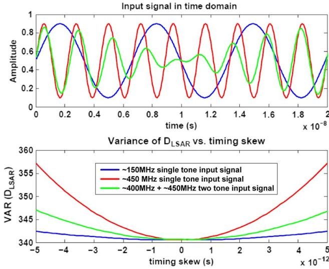
Fig. 10. Behavioral simulation result: Timing skew vs.  $\text{VAR}(D_{LSAR})$ .
