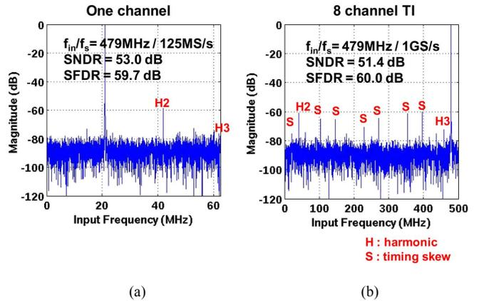
Fig. 18. Measured spectrum after background timing skew calibration: (a) single-channel result and (b) time-interleaved result with a Nyquist rate input signal at 479 MHz.
