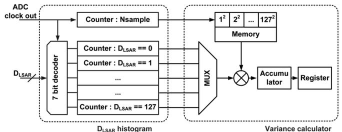
Fig. 14. Block level implementation of timing skew calibration.
