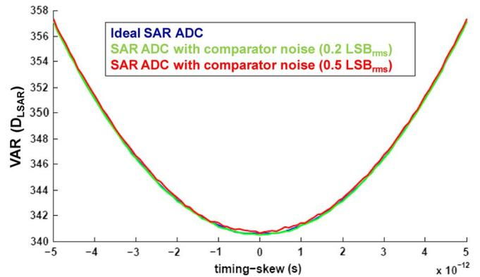
Fig. 13. Behavioral simulation result with comparator noise in SAR ADC.
