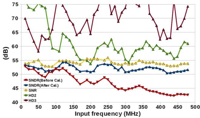
Fig. 20. Measured SNDR/SNR/HD2/HD3 versus input frequency of TI channels.
