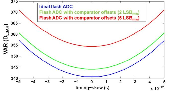
Fig. 11. Behavioral simulation result with comparator offsets in the flash ADC.
