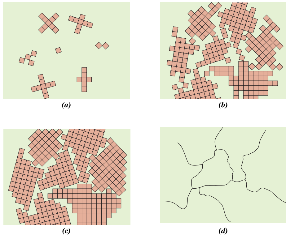
Figure 3.20 Schematic diagrams of the various stages in the solidification of a polycrystalline material; the square grids depict unit cells. (a) Small crystallite nuclei. (b) Growth of the crystallites; the obstruction of some grains that are adjacent to one another is also shown. (c) Upon completion of solidification, grains having irregular shapes have formed. (d) The grain structure as it would appear under the microscope; dark lines are the grain boundaries. (Adapted from W. Rosenhain, An Introduction to the Study of Physical Metallurgy , 2nd edition, Constable & Company Ltd., London, 1915.)
