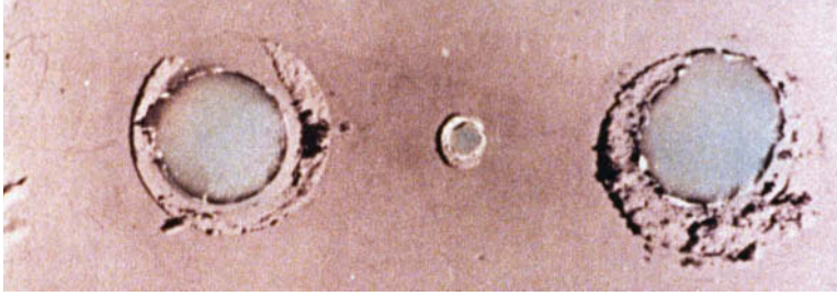
Figure 17.15 On this plate, which was immersed in seawater, crevice corrosion has occurred at the regions that were covered by washers. (Photograph courtesy of LaQue Center for Corrosion Technology, Inc.)
