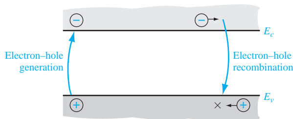
Figure 6.1 | Electron-hole generation and recombination.
