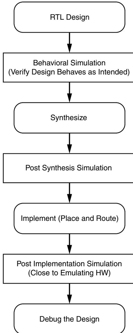
Figure 1-1: Simulation Flow
